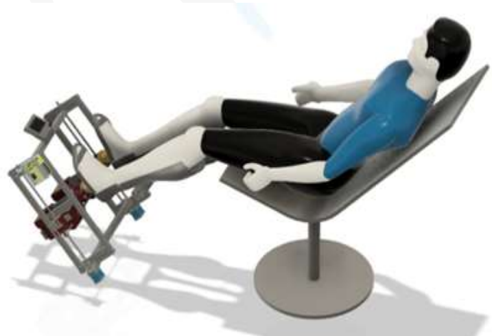
Foot sole massager with adjustable foot length accommodating variation in height of a person.
